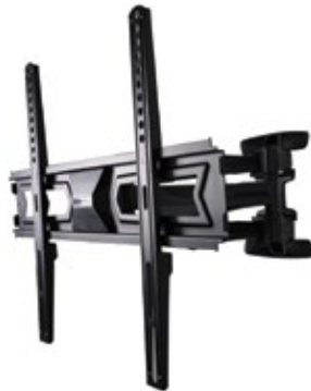
AM50 The AM50 is a dual arm swingout mount for flat panel displays. For use with displays with a VESA mounting pattern of 75 x 75mm to 200 x 200mm. Enables fine tunes vertical adjustment.
